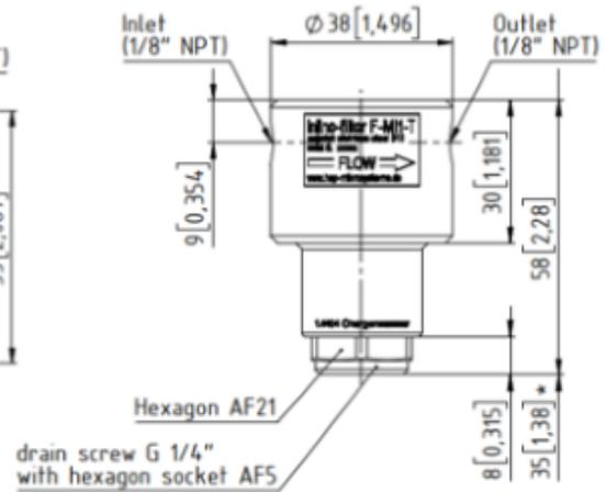
\* Servicing height for filter element exchange
