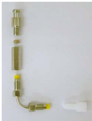
Assembly of the reservoir stainless steel
