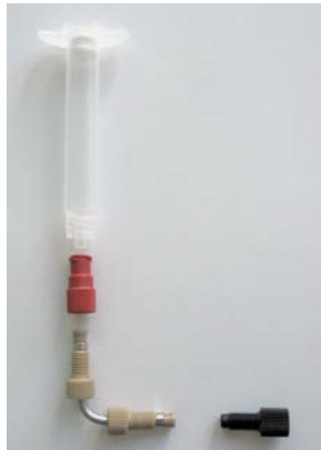
Assembly of the reservoir plastic 3 ml
