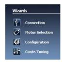
The "Connections" button is always displayed, the other buttons are only displayed if a connection with a drive unit already exists and the respective function is supported by its controller.
