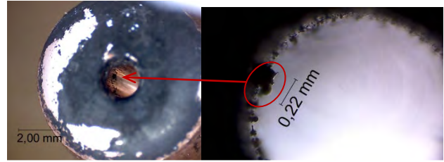
Photo 26: Copper deposits in the contact tip (located about 3 mm deep)
