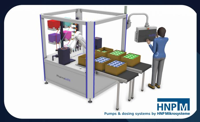
**UNICO** is a modular automation solution for the production of **personalized creams and beauty products.** State-of-the-art robot and control technology paired with precise pumps as well as dosing systems from **HNP Mikrosysteme** make **UNICO** universally deployable. The basic system offers processing of ten different ingredients and can be expanded as desired.
