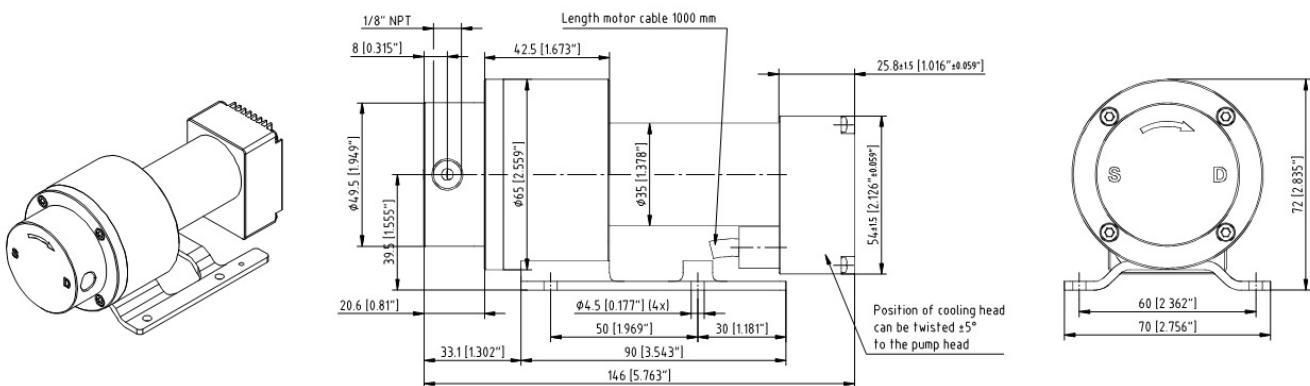
**Dimensions mzl-6355 F (Fluid connection 1/8" NPT internal thread, frontal)**
