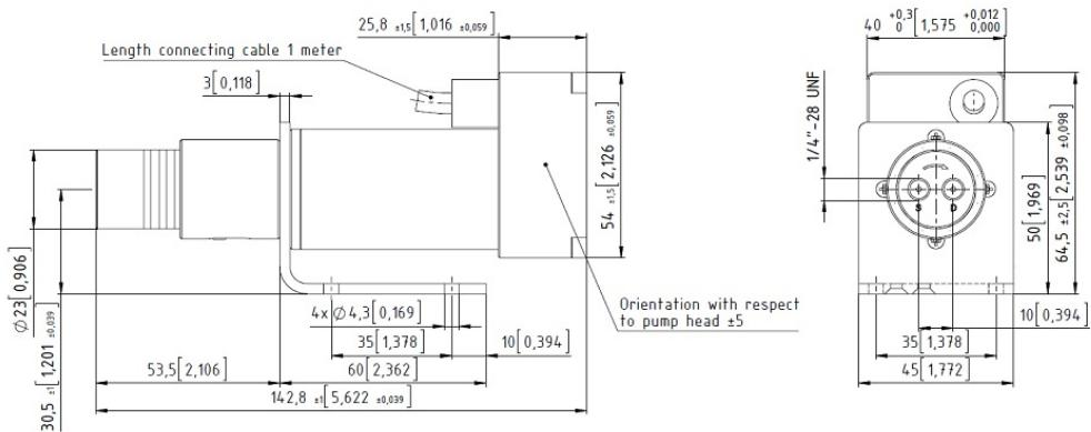
**Dimensions mzl-4005 S/F (Fluid connection 1/4"-28 UNF, frontal; inlet 1/8" NPT internal thread, lateral)**
