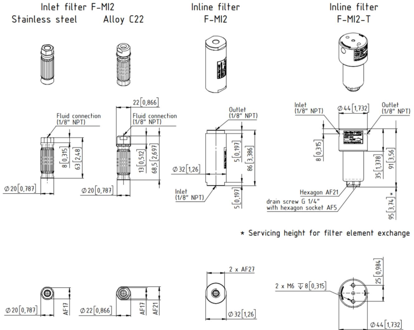
\* Servicing height for filter element exchange
